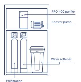
Purify your municipal, well or brackish water at the point of entry to your home. Bluewater Whole House SuperiorOsmosis System helps protect pipes, plumbing fixtures and appliances against sediment buildup and corrosion while providing great-tasting drinking water and clearer, cleaner water for bathing, washing, and laundry throughout your home
