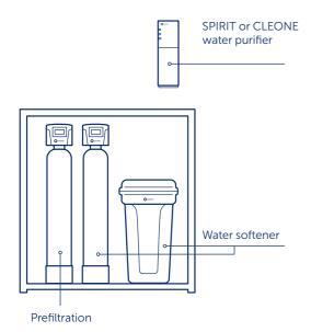
Bluewater Whole House Filtration System is tailored to meet the treatment needs of your water. Bluewater Whole House Filtration System consists of a water softener and a prefiltration module installed at the point of entry into your home and a reverse osmosis water purifier installed under your sink for purified water for your kitchen.
